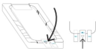
7. Lower glass using "Align" tab to match raised triangle on Tray.
