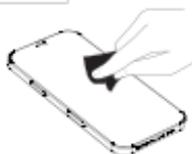
11. Rub screen with Microfiber Cloth to remove any remaining bubbles.
