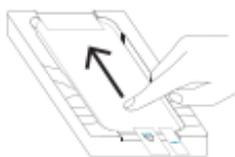
8. Adhere Glass by rubbing finger up center of the Glass.
